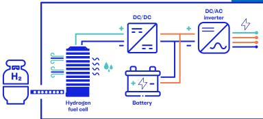
Through an oxidation reaction between hydrogen  $(H_2)$  and the oxygen  $(0_2)$  in the air, the pile produces water  $(H_20)$ ... and electricity. Combined with an inverter and a battery, the generator delivers alternating current, suitable for supplying electricity to customers during work carried out by Enedis or its contractors.
